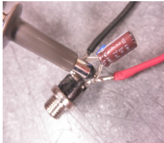
Figure 1: Noise Measurement Caps and Probe with picture of the technique.
