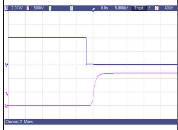
Figure 4: AVO50-48S1V2 typical start-up from CNT on
