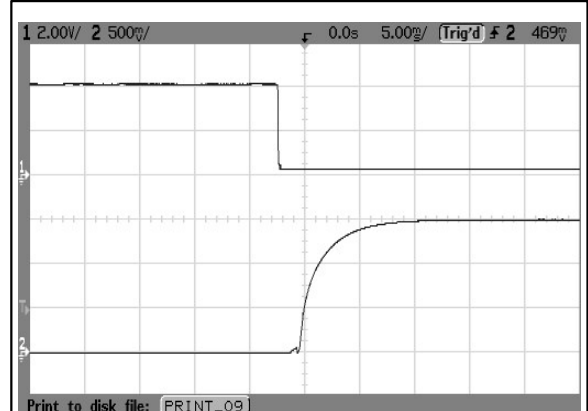
Figure 15: AVO50-48S1V5 typical start-up from CNT on
