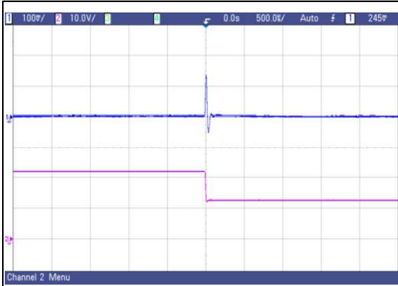
Figure 40: AVO50-48S2V5 Transient Response 50%~25% load change, 1A/uS slew rate, Vin=48V Ch 1: Vo Ch 2: Io
