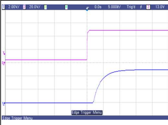
Figure 58: AVO50-48S05 typical start-up from power on
