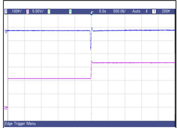
Figure 63: AVO50-48S05 Transient Response 50%~75% load change, 1A/uS slew rate, Vin=48V Ch 1: Vo Ch 2: Io
