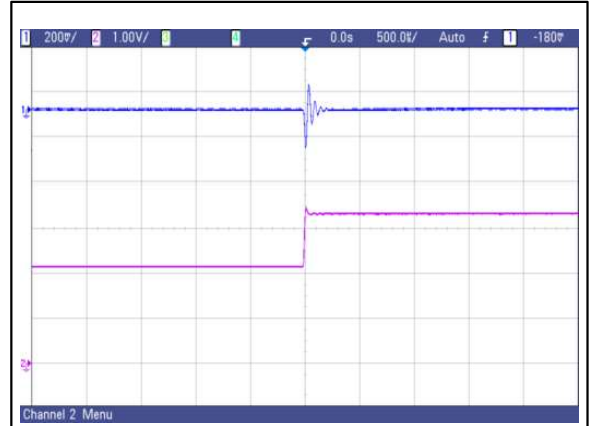
Figure 8: AVO50-48S1V2 Transient Response 50%~75% load change, 1A/uS slew rate, Vin=48V Ch 1: Vo Ch 2: Io
