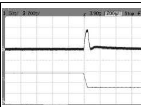
Figure 49: AVO50-48S3V3 Transient Response 50%~25% load change, 0.1A/uS slew rate, Vin=48V
