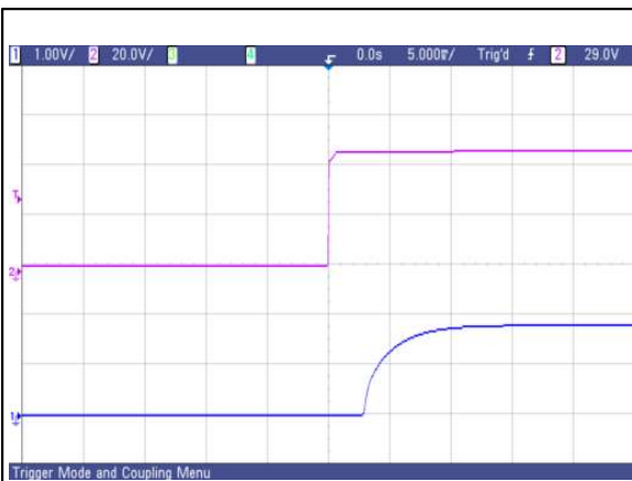
Figure 25: AVO50-48S1V8 typical start-up from power on
