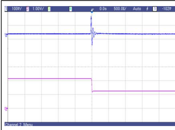
Figure 7: AVO50-48S1V2 Transient Response 50%~25%load change, 1A/uS slew rate, Vin=48V Ch 1: Vo Ch 2: Io
