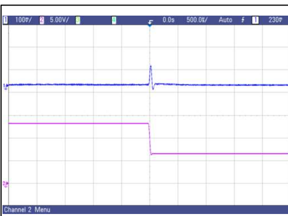
Figure 60: AVO50-48S05 Transient Response 50%~25% load change, 0.1A/uS slew rate, Vin=48V
