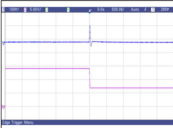
Figure 62: AVO50-48S05 Transient Response 50%~25%load change, 1A/uS slew rate, Vin=48V Ch 1: Vo Ch 2: Io
