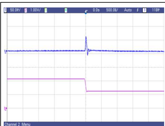
Figure 5: AVO50-48S1V2 Transient Response 50%~25% load change, 0.1A/μs slew rate, Vin=48V
