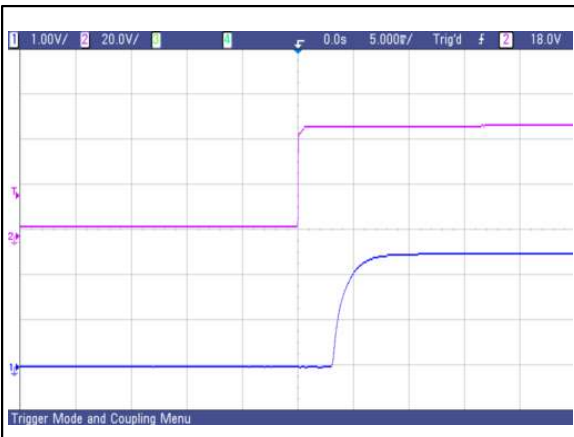
Figure 36: AVO50-48S2V5 typical start-up from power on
