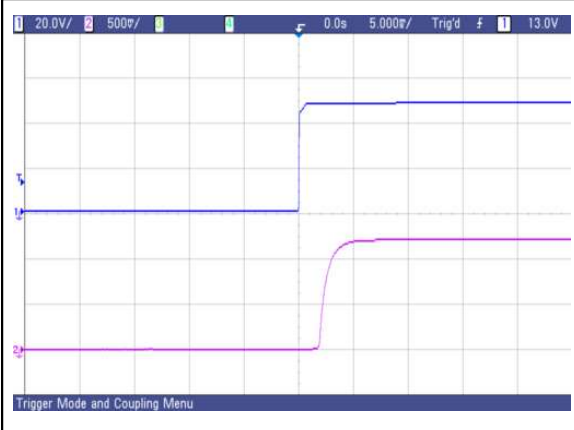
Figure 3: AVO50-48S1V2 typical start-up from power on
