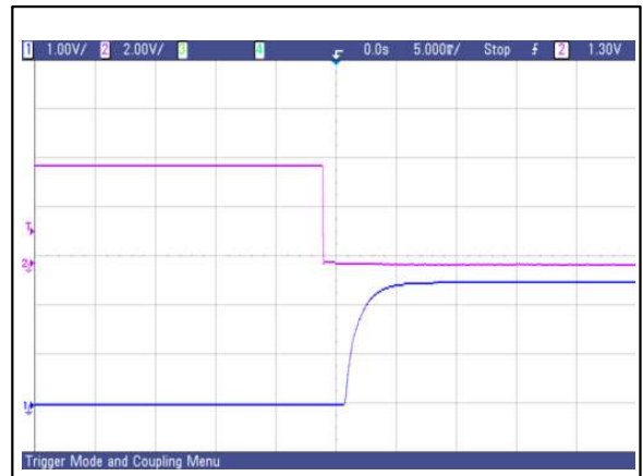
Figure 37: AVO50-48S2V5 typical start-up from CNT on
