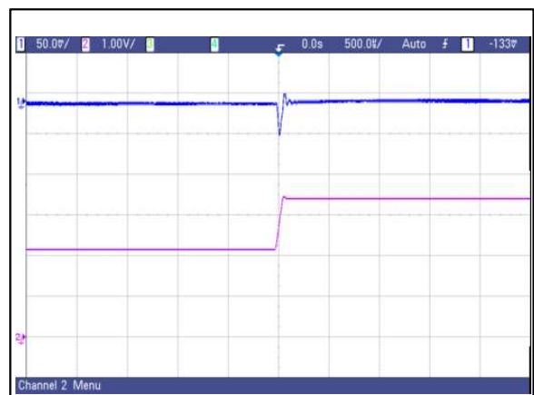
Figure 28: AVO50-48S1V8 Transient Response (500uS/div) 50%~75% load change, 0.1A/uS slew rate, Vin=48V
