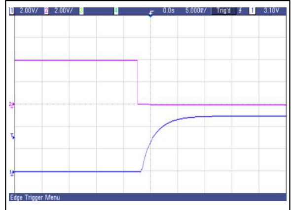
Figure 59: AVO50-48S05 typical start-up from CNT on
