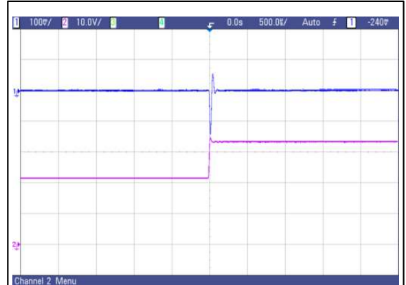
Figure 41: AVO50-48S2V5 Transient Response 50%~75% load change, 1A/uS slew rate, Vin=48V Ch 1: Vo Ch 2: Io
