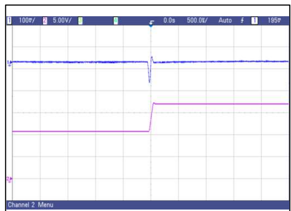
Figure 61: AVO50-48S05 Transient Response 50%~75% load change, 0.1A/uS slew rate, Vin=48V
