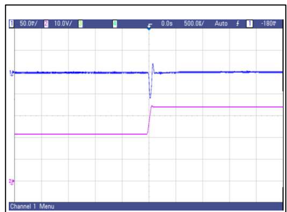
Figure 39: AVO50-48S2V5 Transient Response 50%~75% load change, 0.1A/µs slew rate, Vin=48V
