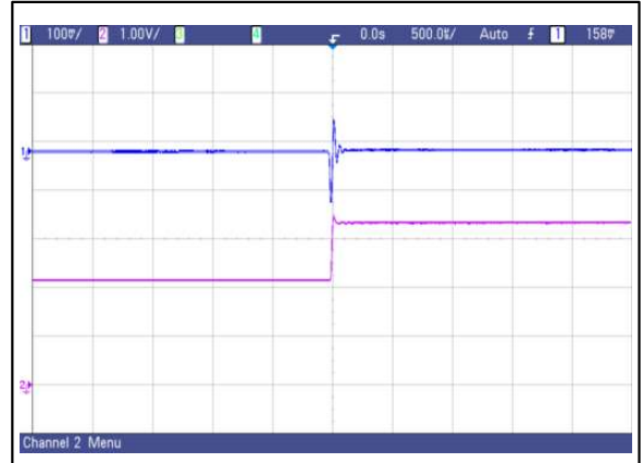
Figure 30: AVO50-48S1V8 Transient Response 50%~75% load change, 1A/uS slew rate, Vin=48V Ch 1: Vo Ch 2: Io
