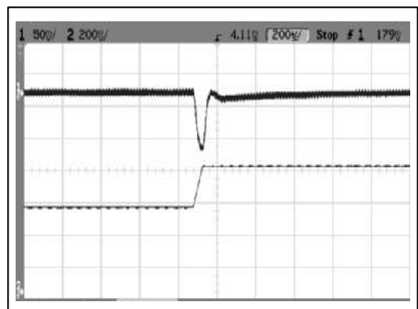
Figure 50: AVO50-48S3V3 Transient Response 50%~75% load change, 0.1A/uS slew rate, Vin=48V
