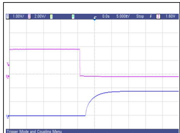
Figure 26: AVO50-48S1V8 typical start-up from CNT on
