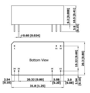
All dimensions in mm (inches) Tolerance: X.X±0.25 (X.XX±0.01) X.XX±0.13 (X.XXX±0.005) Pin pitch tolerance: ±0.25 (±0.01) Pin dimension tolerance: ±0.1 (±0.004)
