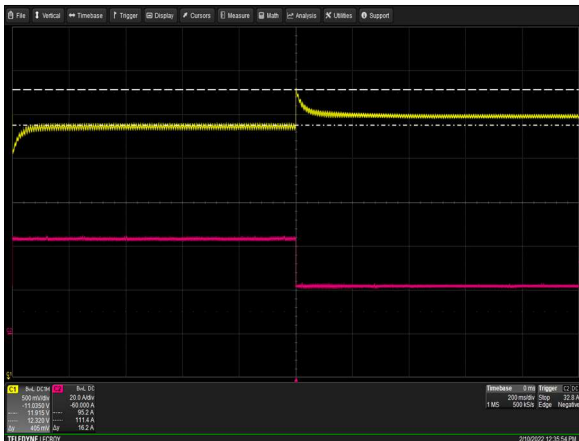
Figure 9: AIF42BAC-01N Transient Response - V O Deviation 100% to 50% load change 1A/μs slew rate Vin = 230Vac Ch 1: V O Ch 2: I O
