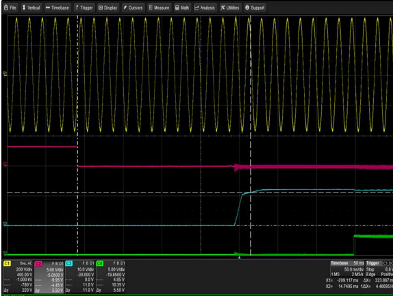
Figure 4: AIF42BAC-01N Turn-On Delay via PSON Vin = 264Vac Load: I O = 42A I SB = 0.25A Ch 1: AC Mains Ch 2: PSON Ch 3: V O Ch 4: PSU-Good
