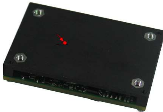
Figure 17 Test point on baseplate
