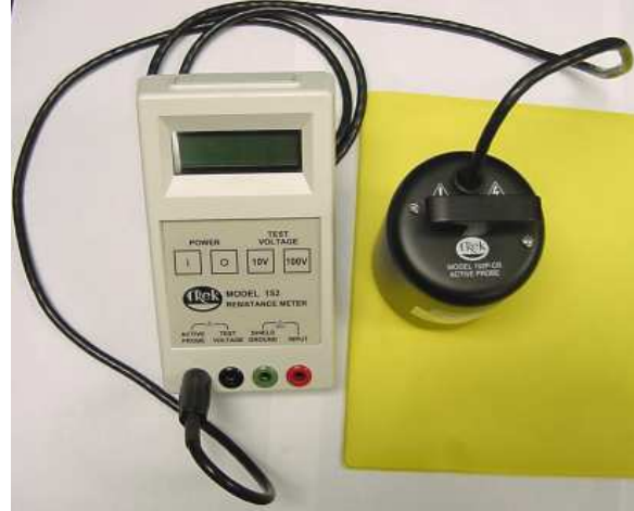
Figure 4: Surface resistivity measurement setup.
