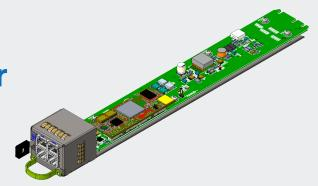
Advanced Energy's Artesyn Power Management Controller (PMC) is a hot-pluggable controller in the shelf that monitors and facilitates the power supply units through a 10/100/1000MB Base-T Ethernet port and can be connected directly to the rack switch.
