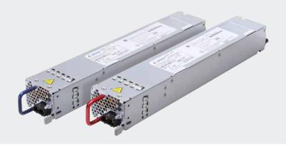
Advanced Energy's Artesyn DS1100TDC series bulk front end DC-DC power supply accepts a wide range -40 to -72 Vdc input and provides a main 12 V output plus a 3.3 V standby output. Housed in an industry standard 1U x 2.1 inch rack-mounting package and able to deliver 1,100W, the power supply is ideal for space-constrained applications. This series comes in two airflow versions – output-connector to input-connector and vice versa.
